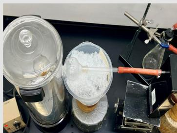
Figure 1. Kugelrohr distillation of a tertiary amide.
