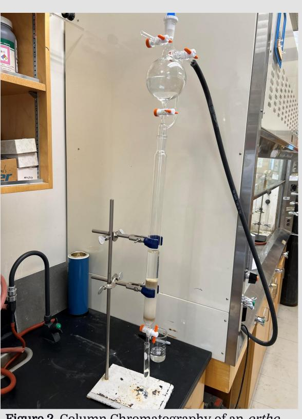
Figure 2. Column Chromatography of an orthometalated product.
